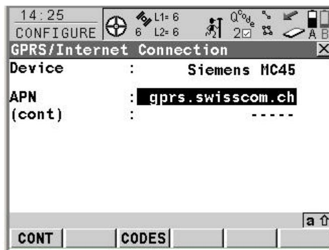
The **APN** can be thought of as the “home page” of the telecom provider using GPRS for accessing the Internet. Contact your telecom provider to get the correct APN name. The following web site gives an overview of the different parameters (APN, User ID, password) for different telecom providers [http://www.access-sys-eu.com/GPRS\\_Settings.95.0.html](http://www.access-sys-eu.com/GPRS_Settings.95.0.html). Note, the accuracy of this information cannot be guaranteed.
