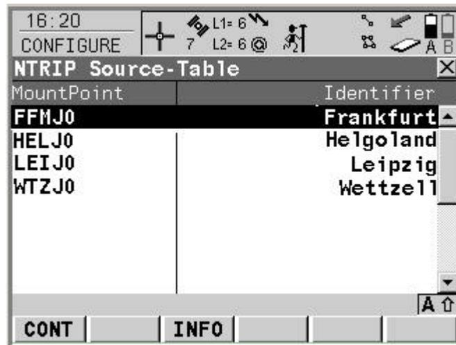
Move the focus to the required Mountpoint and press **F1(CONT)** to copy the Mountpoint name to the **Mountpnt** prompt in the **NTRIP** page of the **CONFIGURE Additional Rover Options** panel.
