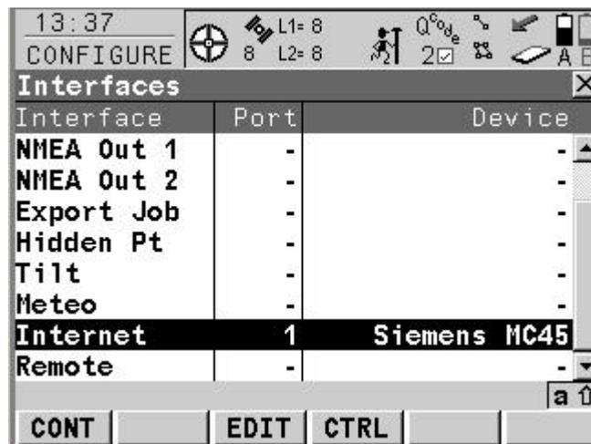
Access the **CONFIGURE Interfaces** panel, place the focus on the Internet Interface and press the **F3(EDIT)** button to access the **CONFIGURE Internet Interface** panel. The Interface specific parameters can now be configured.
