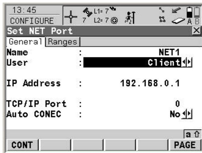
As already mentioned, when using GPRS to access the Internet it is only possible for the sensor to act as a TCP/IP Client due to the dynamic IP address of the sensor. Therefore set the **User** prompt to **Client** and enter the **IP Address** of the Server (Broadcaster) to where the Net port should connect.
