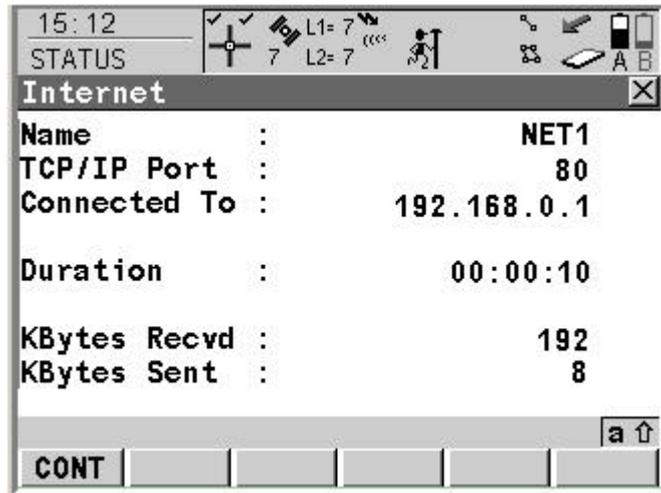
The **STATUS Internet** panel shows the **Duration** of the connection for the individual Net port from the time the connection is established till the moment the Net port is disconnected from the Server. Also shown is how much data is sent or received in that time period.
