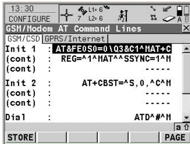
In the **CONFIGURE GSM/Modem AT Commands** panel, two pages are available.
