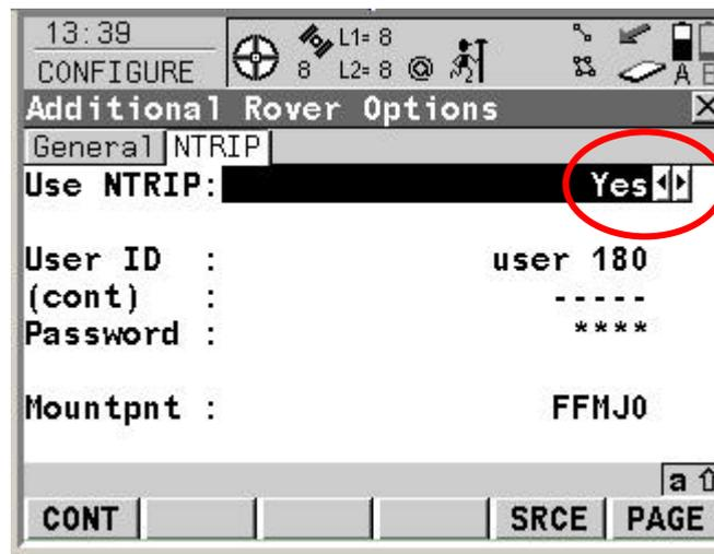
The **Use NTRIP** prompt allows the sensor to be configured to receive RTK data via NTRIP. Set this prompt to **Yes** and configure the NTRIP relevant settings.
