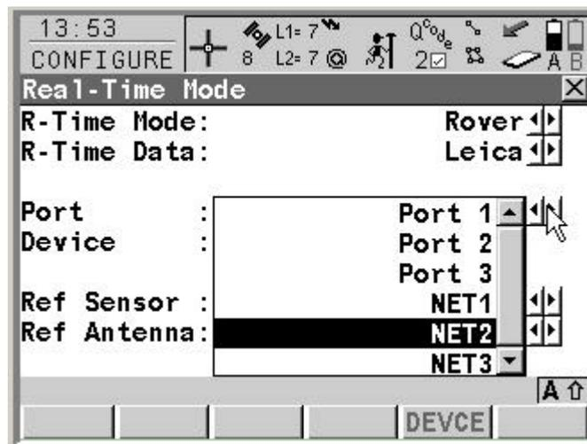
Note, these new ports should be treated in the same way as the “normal physical” ports (Port1, Port2 and Port3) – this means that only one port is allowed to be used with one Interface.
