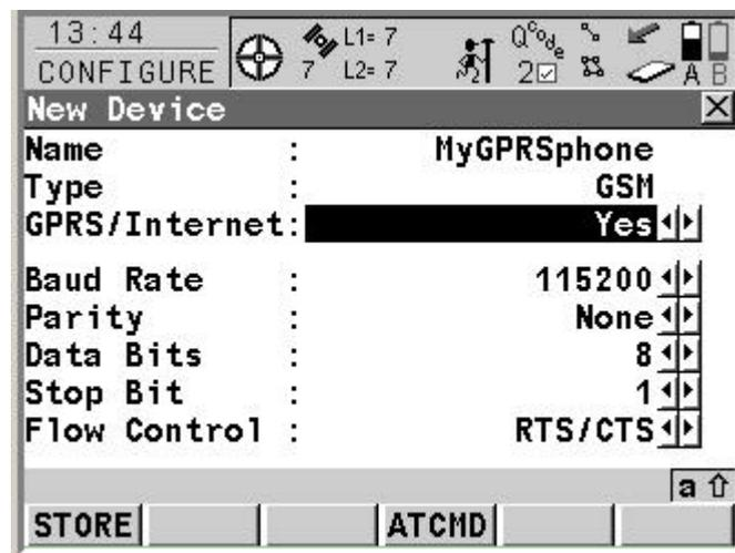
Select **Yes** at the new **GPRS/Internet** prompt. This informs the sensor that this device is GPRS capable and allows AT commands to be entered which will steer the GPRS functionality of the device. The
