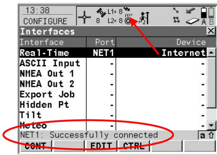
RTK data would now be received from the Server (e.g. the NTRIP Caster) and the RTK arrow would flash to indicate RTK data being received.
