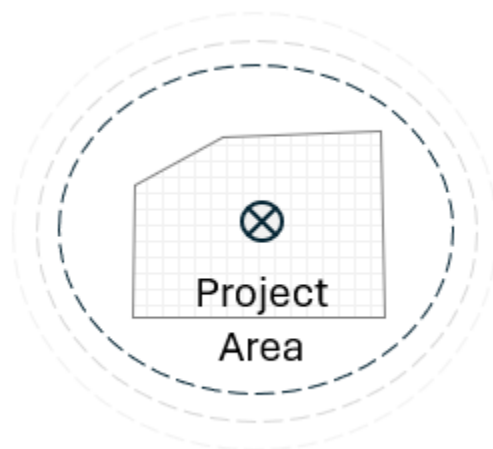
Figure 1 – Single control point (radial). Suitable only for small project sites.
